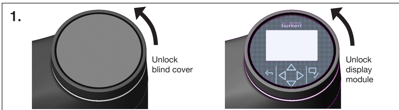
Fig. 31: Remove blind cover or display module
