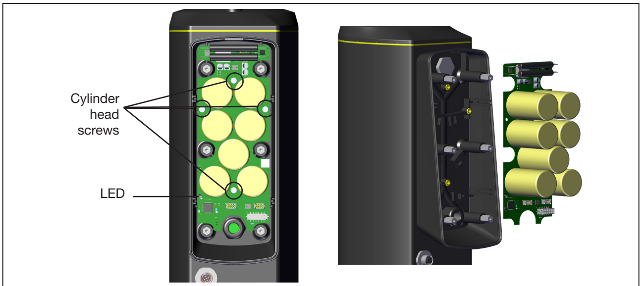
Fig. 15: Loosen screws on the printed circuit board/remove SAFEPOS energy-pack
