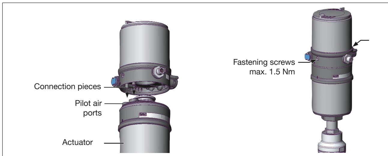
Figure 22: Installation of positioner, series 2103, 2300 and 2301
