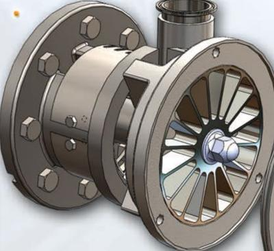
Tight manufacturing tolerances and the unique vane-shaped impeller enable the SP to handle shear sensitive products efficiently.
