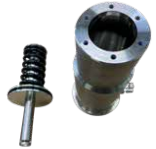
FIG. 8 - PISTON, SPRING, AND ACTUATOR STEM REMOVED
