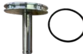
FIG. 28 - ACTUATOR CYLINDER, SPRING ASSEMBLY AND PISTON ASSEMBLY REMOVED
