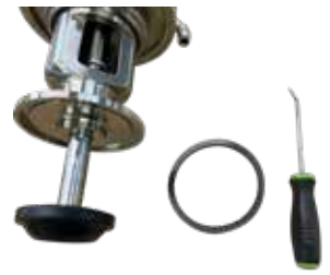
FIG. 10 - GASKET REMOVED TO BE REPLACED
