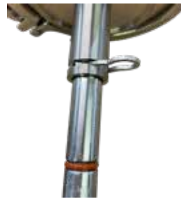
FIG. 15 - SPRING CLIP HALFWAY REMOVED OR INSTALLED
