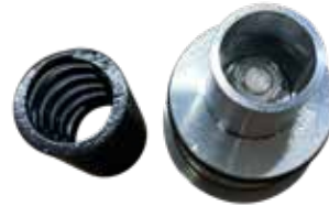
FIG. 10 - SPRING CLIP AND PLUG AND STEM REMOVED
