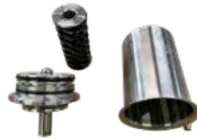
FIG. 24 - ACTUATOR CYLINDER, SPRING ASSEMBLY AND PISTON ASSEMBLY REMOVED
