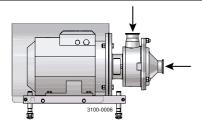
Avoid damaging the inlet and the outlet.
