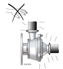
**Never** stick your fingers or any tool through the adaptor or the drain hole in the pump casing when the pump is running.
