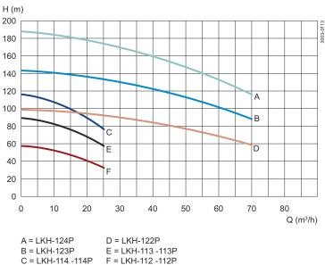
Frequency: 50Hz - Speed (synchr): 3000 rpm
