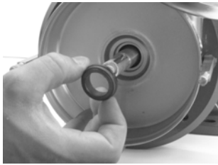
Fig. 23 Stationary ring of the mechanical seal
