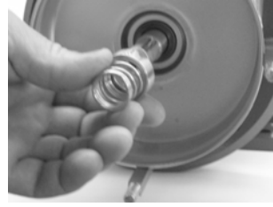
Fig. 22 Rotary ring of the mechanical seal
