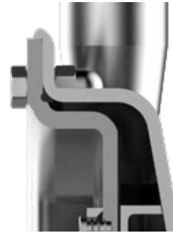
O-ring sealing between pump housing and cover
