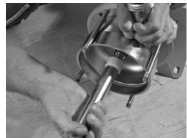
Fig.28: Fixed ring of the mechanical seal and discharge casing
