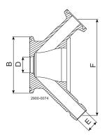
Figure 3. Valve body: Clamp
