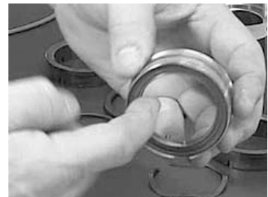
Fig.48: Seal carrier of the flushed mechanical seal
