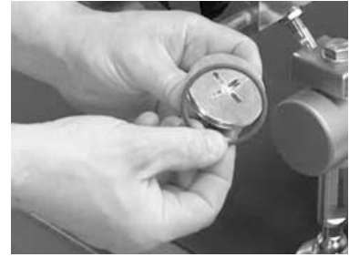
Fig.62: Rotor bolt, O-ring
