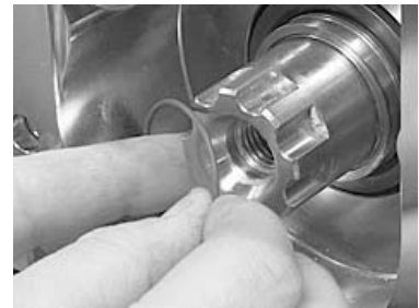
Fig.55: O-ring, seal carrier
