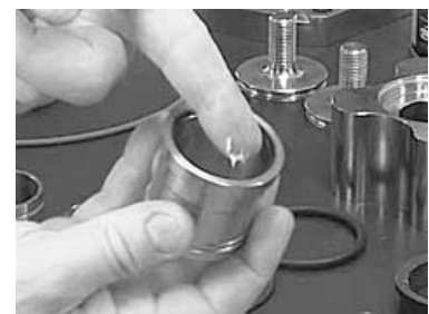
Fig.45: O-ring, shaft protection sleeve
