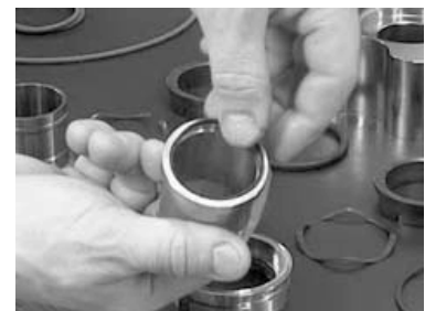
Fig.44: O-ring, shaft protection sleeve
