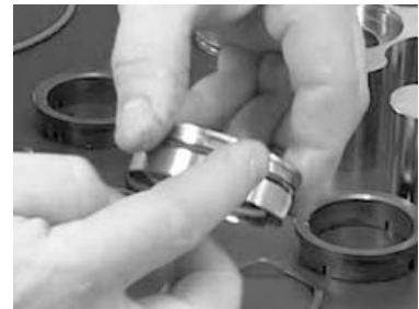
Fig.47: O-ring, seal carrier
