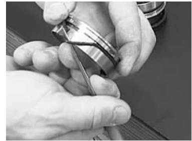
Fig.42: O-ring, radial packing ring
