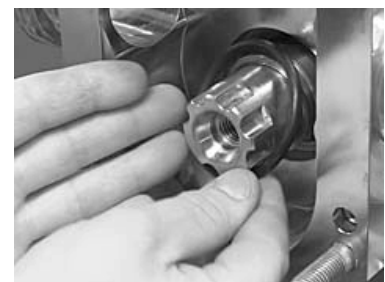
Fig.53: O-ring, drive shaft
