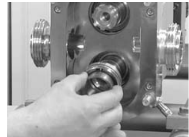
Fig.51: Mechanical seal, drive shaft
