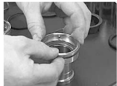
Fig.49: Seal carrier, shaft protection sleeve
