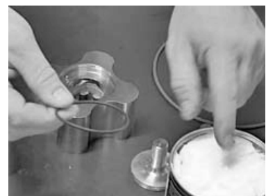
Fig.57: O-ring, drive, sealing surfaces
