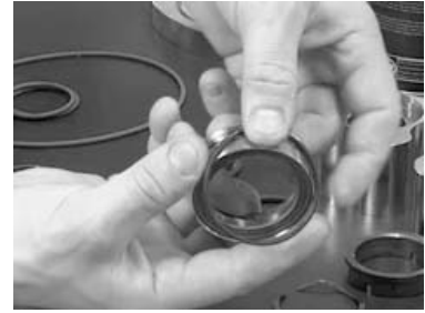
Fig.46: O-ring, seal carrier
