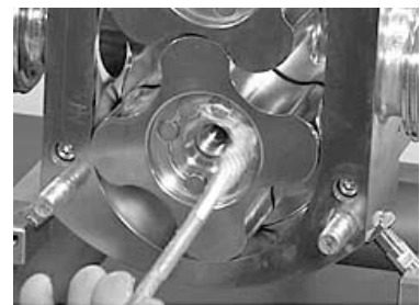
Fig.61: Contact surface rotor/rotor bolt
