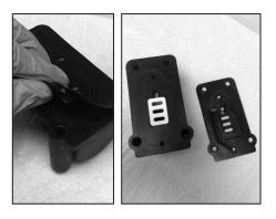
STEP 3 Remove the "Air-Valve Gasket" from the main "Air-Valve Assembly".
