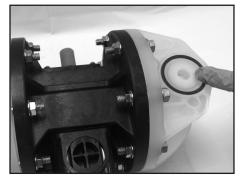
STEP 5 Remove the "Suction Manifold".
