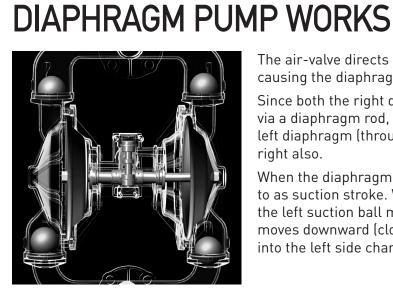
The air-valve directs pressurized air behind the diaphragm on the right, causing the diaphragm on the right to move outward (to the right).
