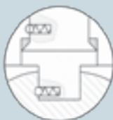
Pyramidal Stem, Double Sealing & Anti-Static Device (Optional)
