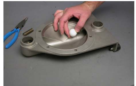
Remove the valve stops [3] and the ball valves [15] out of the side housings [1]. For the G125 and G200 the use of a screwdriver to remove the valve stops maybe is more convenient.
