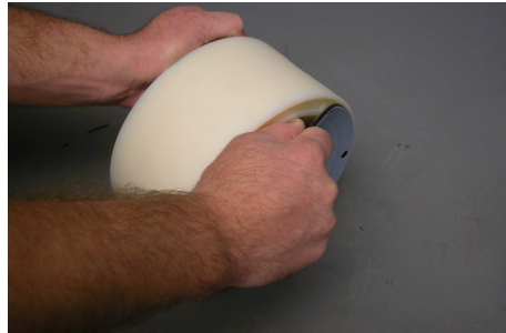
Screw one diaphragm [14] counter clockwise off the shaft [13].
