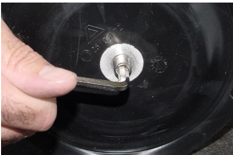
Screw out the set screws, shaft [13a].
