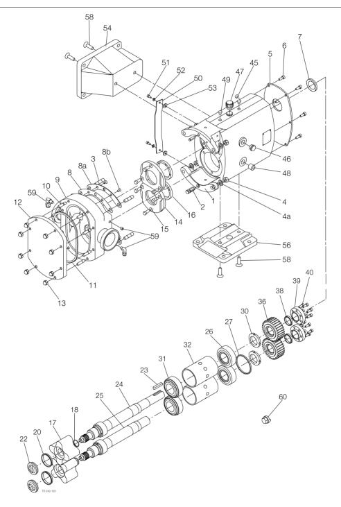
The drawing shows exploded view of the SX1 - 3 pump range. The drawing includes all items of the pump.
