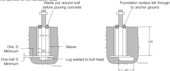
The drawing above shows two typical methods for foundation bolt retaining. The sleeve allows for "slight" lateral movement of the bolts after the foundation is poured. Rag or waste paper can be used to prevent the concrete from entering the sleeve while the foundation is poured. A minimum of 14 days us normally required to allow the curing of the concrete prior to pump unit installation.
