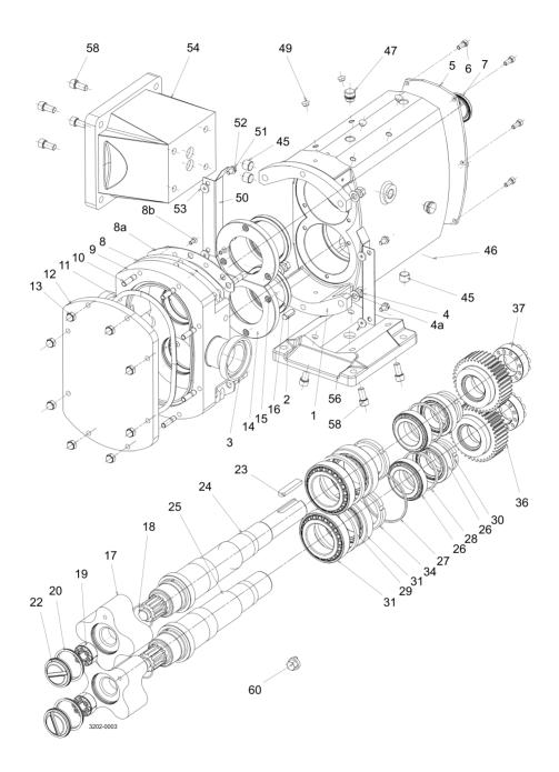
The drawing shows exploded view of the SX6-7 pump range. The drawing includes all items of the pump.
