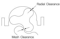
Front Clearance Rotor Length Bac Minimum mesh clearance at any mesh position. All dimensions in millimeters
