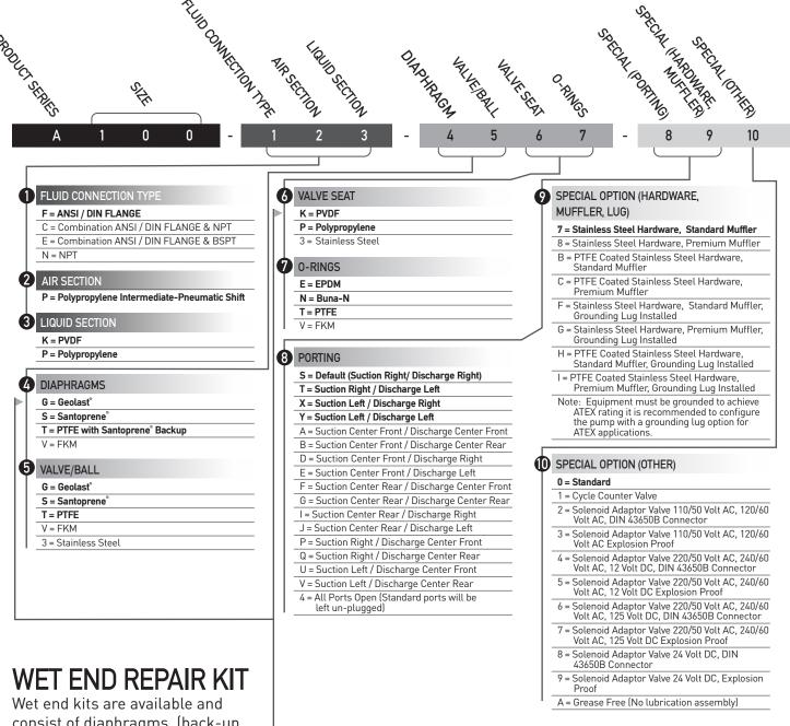
Wet end kits are available and consist of diaphragms, (back-up diaphragms if required), balls, seats and seat 0-Rings.
